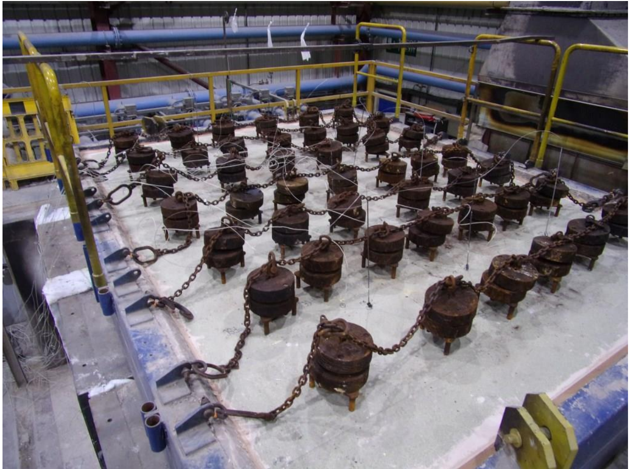
Unexposed face before test.
